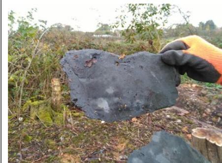
Two types of slate were at the cottages. The Welsh slates are purple and thin, the quality of the slate allows it to be cut very thinly. This makes it popular with builders as they can use less wood in the roof structure.
