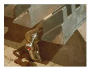
The holes in the castings which enabled them to be bolted onto the wooden wheel were ideal for attaching the chain and shackle.
