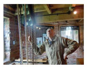
The weight and shape of the casting put a distortion on the chain hoist and periodically the system jammed. This required careful communication between the floors to ensure that the correct chains were pulled to release the jam.
