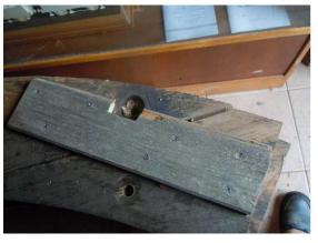
Even four year old seasoned oak can crack, so a temporary patch was added to keep this segment in one piece. After it was fitted on the wheel the patch was removed as the bolts held it in place.
