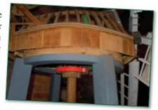
and transfers the wind power generated by the sails to the drive shaft so as to operate the mill's machinery.
