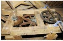
Inside the cap, the drive shaft turns a number of gears.
