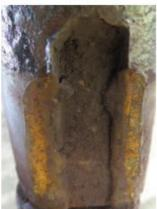
The keyway in the exterior drive shaft was damaged and the shaft sections were out of alignment. A new muff coupling had to be made and fitted.
