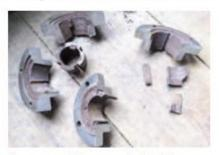
Once removed the reason for the failure was apparent as it was in several pieces.
