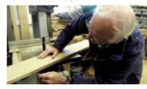
"Biscuit holes" were made along the joining edges so that "biscuits" (small wooden discs) could be used to seamlessly join each piece to its neighbours. Gradually each sail took shape.
