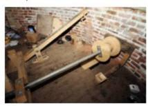
The winding drum is on an axle.
