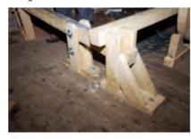
When the miller pulls on the rope to operate the hoist, the rope pulls the free end of the control lever down. This raises the hinged end of the control lever, thereby raising the lifting beam.
