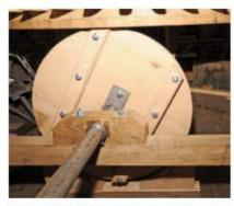
Raising the lifting beam also raises the drive wheel to the bottom of the wallower. This creates a friction drive in which the wallower turns the drive wheel.
