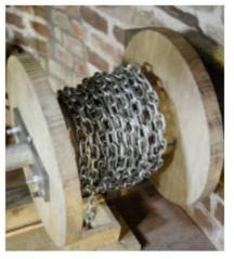
A gentle tug on the rope will lower the chain until sufficient chain has been unwound to enable the weight of the chain to take it down to the Meal Floor.
