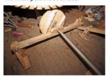
The opposite end of the axle passes over the lifting beam and is attached to the wooden drive wheel.
