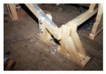
When the hoist is at rest, the control lever is angled downwards underneath the lifting beam.
