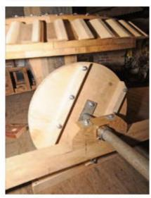
The default position of the drive wheel is a couple of finger widths below the wallower.
