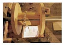
The chain is attached to a winding drum, which is positioned above the trap doors in the cap.
